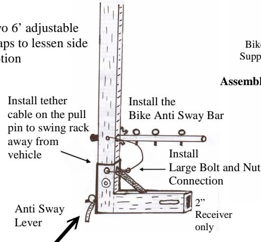
Tighten the lever clockwise to engage the patented "No Wobble" system, which will eliminate the movement of the insert tube in the receiver. The lever should be turned "up" or to the side after tightening to prevent it from being damaged in the case you have to descend a steep driveway or have some other close encounter with "Solid Ground." The rack should now be attached to your vehicle, and locked into place.
