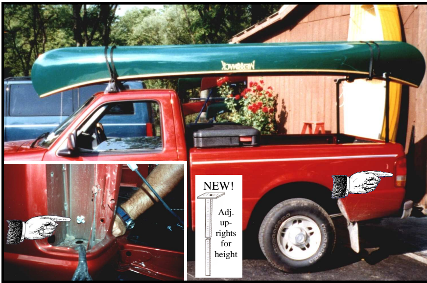
Shown: Installed Nutsert Above: Style #1 rear rack and a half set Yakima "Q" tower front.
