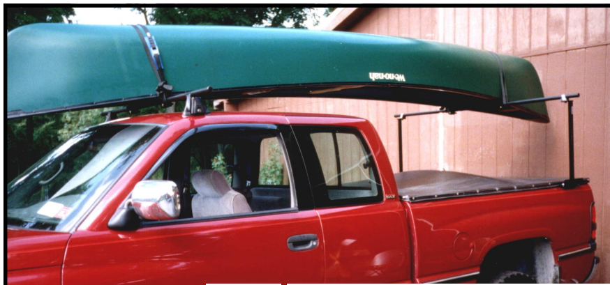
Shown: Installed Nutsert Above: Style #1 rear rack and a half set Yakima "Q" tower front.
